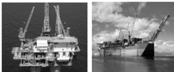
Fig. 1. Kinds of offshore structures: tension leg platform (TLP) and FPSO.
