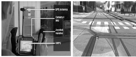
Fig. 2. Virtual redlining for civil engineering: ultra-mobile personal computer (UMPC) (left) and system demonstration (right).
